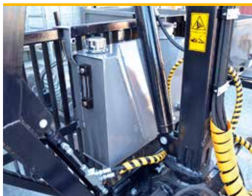
PTO pump and hydraulic tank
